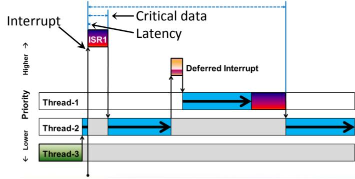
When the interrupt occurs the ISR is activated and will read the hardware registers. The ISR can't communicate with the RTOS so it will defer that operation. This architecture outperforms the unified architecture in latency and reads critical data faster. The RTOS will queue the data for the deferred operation so it has no negative impact on performance.
