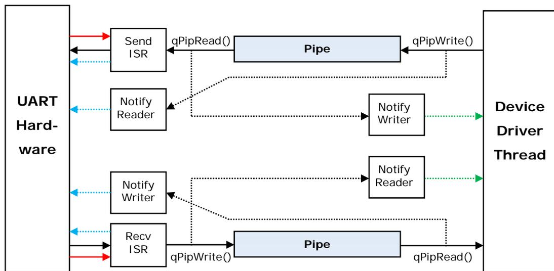
On the left side are the UART hardware registers and on the right side is the thread that functions as a driver. There is a pipe for sending information and a pipe for receiving information. The two ISRs on the hardware side are handling interrupts (red-line). The blue lines set hardware registers and the green lines ready the thread. The solid lines specify how data moves.
