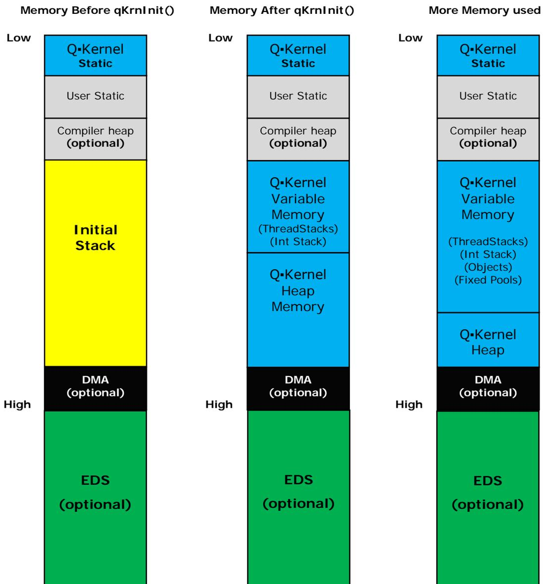
Q-Kernel™ will only use a very small amount of static memory because it will allocate most of its memory requirements dynamically. User static variables will be allocated in User Static memory. Access to this kind of memory must be synchronized with critical sections or mutexes. The DMA and compiler heap are optional.
